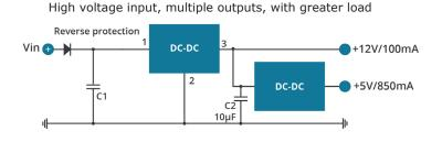
1. The input current amount of the back-grade regulator and the pre-class load should be less than or equal the max load current of the pre-class regulator.
