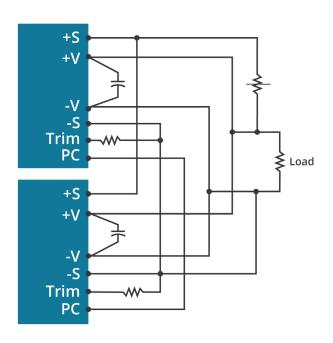
Figure 3 N+1 Redundant Connection
