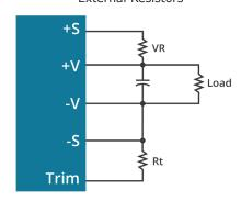
Figure 6 External DC Voltage
