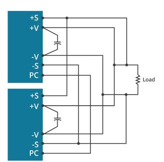
Figure 2 Parallel Connection With Programmed And Adjustable Output
