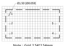
Note: Grid 2.54\*2.54mm Recommended PCB Layout Top View
