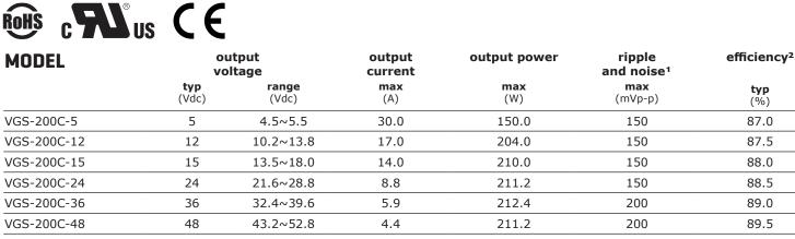
Notes: 1. Ripple and noise are measured at 20 MHz BW with 47 uF aluminum electrolytic capacitor and 0.1 uF ceramic capacitor on the output. 2. Measured at 230 Vac.
