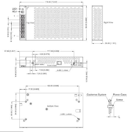
Note: At least one position (1)~ (8) must be securely connected to the GND. (1)
