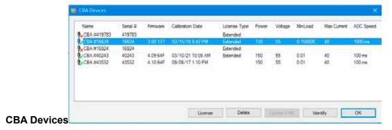
This is a list of the CBA devices known to this software installation. The green check mark indicates units that are currently plugged in to the PC. The units marked **Extended** can use the extended features. To enable extended features, click on a the line marked **CBA** and then click on **License** in the bottom of the window to be prompted for a name and key. Enter the key exactly as provided.
