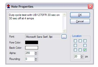
The note properties screen allows for typing the text to be displayed, as well as the location and distance (px) to where the text will be placed, relative to the line data point you selected.
