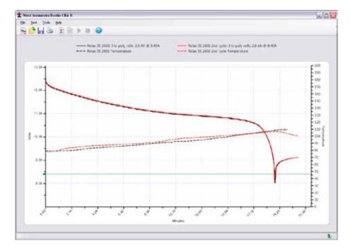
The test will be stopped when the temperature is above the specified threshold or a "Recovery Time" (Discharge Test) can be specified. When the battery reaches the threshold temperature, the test will stop for the given recovery time and then resume. To see the results over time for battery temperature cool down and voltage recovery, use a Voltage versus minutes graph, not Amphrs or Watthrs.
