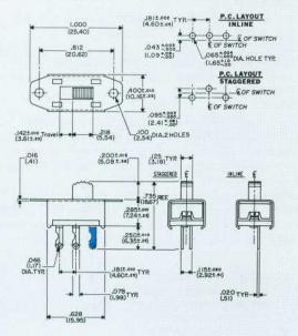
NOTE: SPST versions have one end terminal (shown in blue) removed. Provision for varying current and voltage rating is made by changing internal contact materials.
