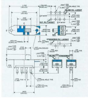
Drawing shows button in extreme right position where LONG detent plate covers topside opening to the left of the button and extends beyond (in blue) housing on right. Specify G-127L or G-128L with suffix indicating current requirement. If topside opening need not be covered, specify G-127S or G-128S with appropriate suffix.
