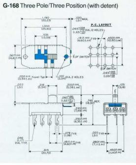
Drawing shows button in extreme right position where LONG detent plate covers topside opening to the left of the button and extends beyond (in blue) housing on right. Specify G-168L with suffix indicating current requirement. If topside opening need not be covered, specify G-168S with appropriate suffix.
