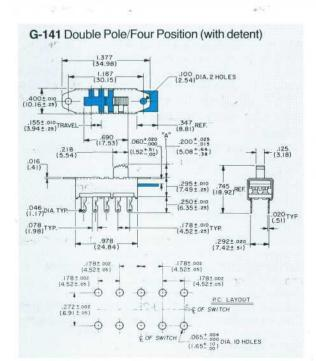
Drawing shows button in extreme right position where LONG detent plate covers topside opening to the left of the button and extends beyond (in blue) housing on right. Specify G-141L with suffix indicating current requirement. If topside opening need not be covered, specify G-141S with appropriate suffix.
