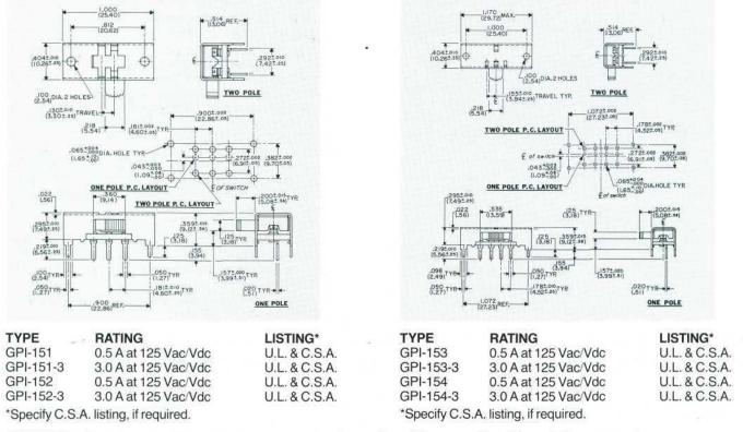
**TOPPERS** – Control panel styling and appearance can be changed by adding an auxiliary "Topper". See page 12. **BUTTONS** – .200" (5.08 mm) button length shown is standard. Other lengths available are .328" (8.33 mm) and .453" (11.51 mm). **MOUNTING** – Plug directly into PC board having suggested hole pattern shown. **SOLDER SHIELD** – Vulcanized fiber shield .020" thick may be shipped assembled or separate as requested.
