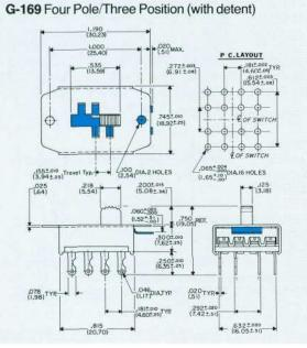
Drawing shows button in extreme right position where LONG detent plate covers topside opening to the left of the button and extends beyond (in blue) housing on right. Specify G-169L with suffix indicating current requirement. If topside opening need not be covered, specify G-169S with appropriate suffix.
