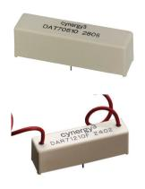
Very high isolation voltages - up to 15kV are achieved through the use of high vacuum reed switches with either rhodium or tungsten contacts which make these relays suitable for high reliability applications, such as cardiac defibrillators, test equipment and high voltage power supplies.
