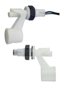
The RSF10 series drop float has been designed to eliminate problems associated with limescale build up around the pivot point of a conventional float switch. It is also suitable in more viscous liquids, that might affect the pivot action of a standard float type. This particular series is primarily for applications where a high level condition has to be monitored.
