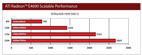
Note 1. e/m indicates the 3D engine (e) and memory (m) clock speed in MHz.
