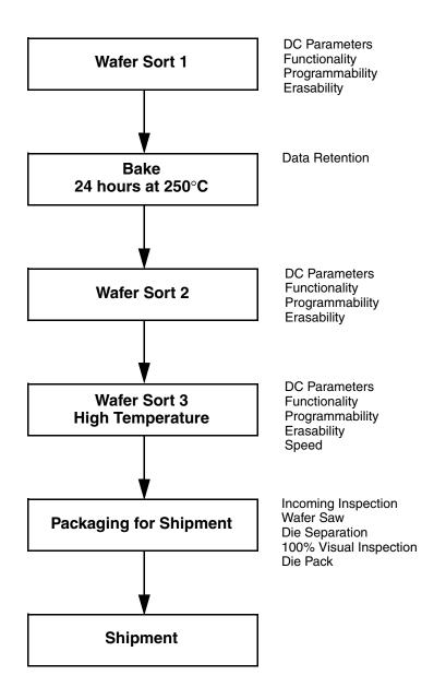
Figure 1. AMD KGD Product Test Flow
