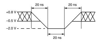
Figure 6. Maximum Negative **Overshoot Waveform**
