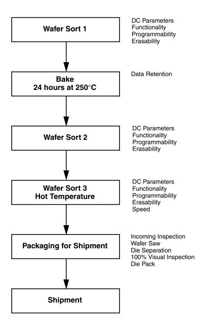
Figure 1. AMD KGD Product Test Flow
