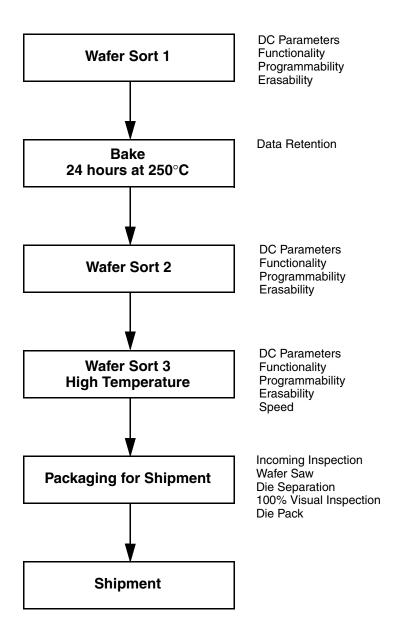
Figure 1. AMD KGD Product Test Flow
