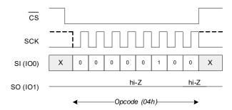
Figure 11. WRDI Bus Configuration in DPI Mode
