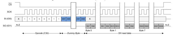
Figure 98. Read Serial Number (RDSN) in DPI Mode
