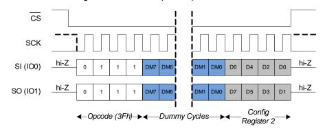
Figure 27. Read CR2 (RDCR2) in QPI Mode
