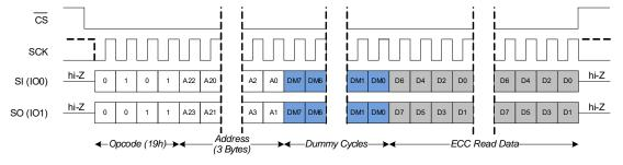
Figure 75. ECC Read (ECCRD) in QPI Mode
