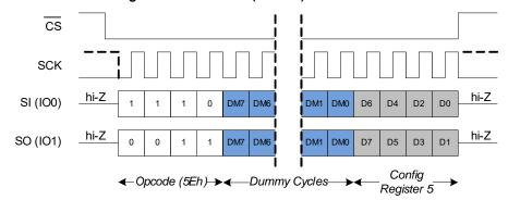
Figure 33. Read CR5 (RDCR5) in QPI Mode
