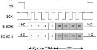
Figure 15. WRSR in QPI Mode (WREN not shown)
