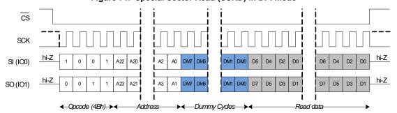
Figure 72. Special Sector Read (SSRD) in QPI Mode
