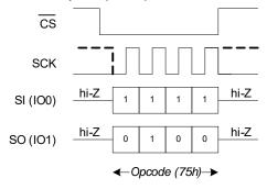
Figure 84. Suspend (EPCS) in QPI Mode
