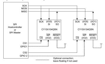
Figure 4. System Configuration with QSPI Port
