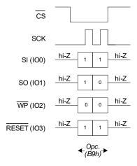
Figure 103. DPD Exit in SPI Mode
