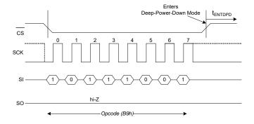
Figure 101. Deep Power-Down Mode Operation in DPI Mode
