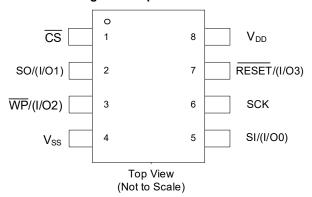
Figure 2. 8-pin GQFN Pinout
