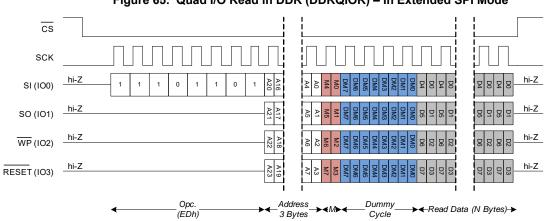
Figure 65. Quad I/O Read in DDR (DDRQIOR) - In Extended SPI Mode
