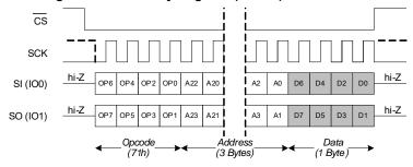
Figure 36. Write Any Register (WRAR) in QPI Mode
