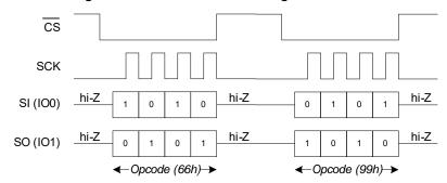
Figure 109. Software Reset Timing in QPI Mode
