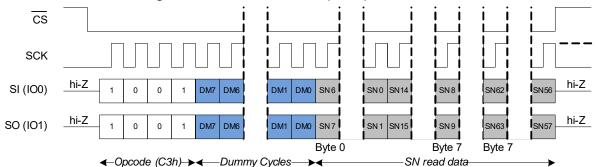
Figure 99. Read Serial Number (RDSN) in QPI Mode
