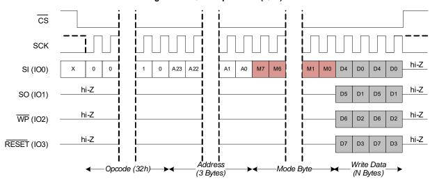
Figure 49. Quad Input Write (QIW)
