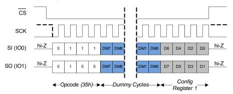
Figure 24. Read CR1 (RDCR1) in QPI Mode
