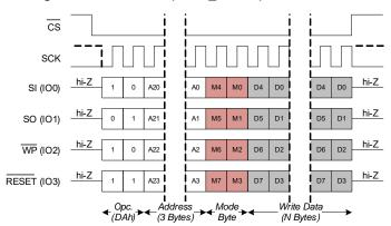
Figure 46. Fast Write (FAST\_WRITE) in QPI Mode
