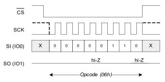
Figure 8. WREN Bus Configuration in DPI Mode
