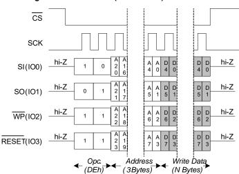
Figure 43. DDR Write (DDRWRITE) in QPI Mode
