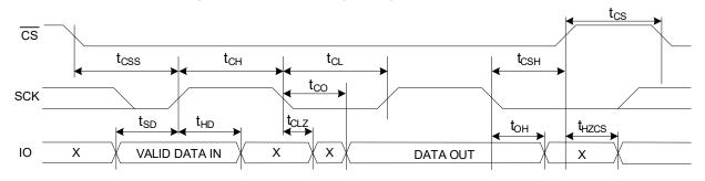
Figure 117. Chip Deselect (CS HIGH) - t<sub>CS</sub> Timing
