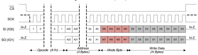
Figure 48. Dual I/O Write (DIOW)
