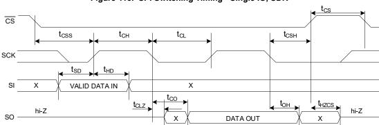
Figure 115. SPI Switching Timing - Single IO, SDR
