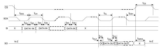
Figure 119. SPI Switching Timing - Multiple I/O, DDR [24]
