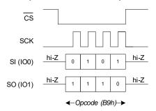
Figure 102. Deep Power-Down Mode Operation in QPI Mode
