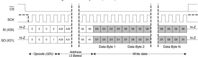
Figure 41. Memory Write (WRITE) in DPI Mode
