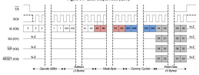
Figure 61. Quad Output Read (QOR)
