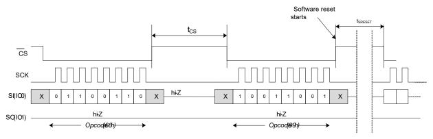
Figure 108. Software Reset Timing in DPI Mode
