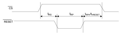
Figure 111. RESET Timing - SPI with QUAD clear (CR1[1]= '0') and QPI disabled (CR2[6] = '0')
