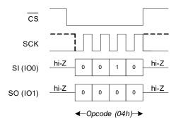
Figure 12. WRDI Bus Configuration in QPI Mode
