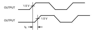
Figure 4. Input-Output Propagation Delay
