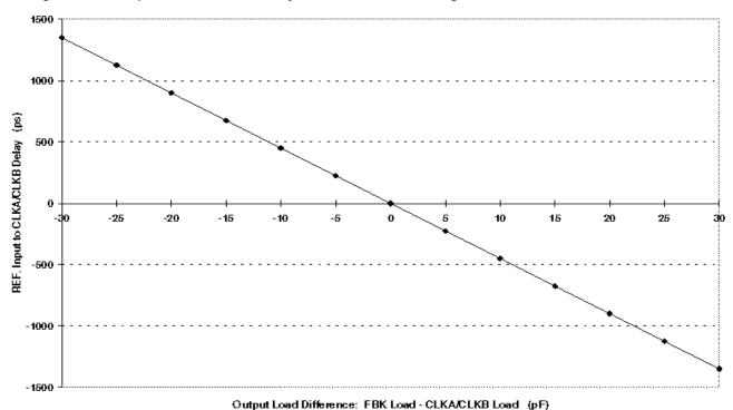
To close the feedback loop of the CY2304, the FBK pin can be driven from any of the four available output pins. The output driving the FBK pin is driving a total load of 7 pF, with any additional load that it drives. The relative loading of this output (with respect to the remaining outputs) can adjust the input-output delay. This is shown in Figure 2.
