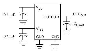
Test circuit for all parameters
