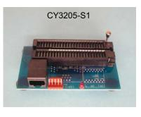
To accommodate the largest number of pin counts with each board, the largest socket is installed. For example, the CY3205-S1 includes a 48-pin DIP socket. It therefore supports 8, 20, 28, and 48-pin DIP parts. The CY3205-S3 includes a 28-pin SSOP socket that can accept both the 20 and 28-pin SSOP parts. The body width of the 48-pin SSOP package is wider than the 20 and 28-pin so the CY3205-S4 is necessary for the 48-pin SSOP parts.
