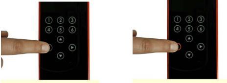
Button does not glow if pressed for less than the time set in the Debounce parameter settings
