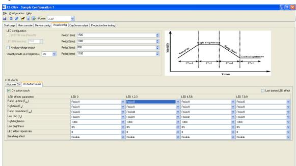
Figure 3-19. Button Controlled LED Effects Enabled
