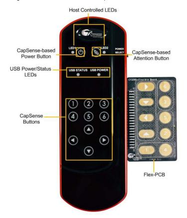
Figure 3-1. CY8CMBR2110 CapSense Controller Kit with Flex-PCB
