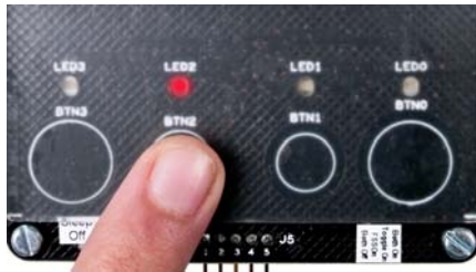
1. Touch a button; the LED turns on
