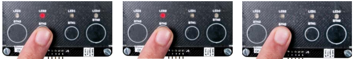
Figure 3-20. Test Sequence for ARST Feature
