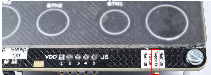
Figure 3-3. Switch Position for Toggle Feature
