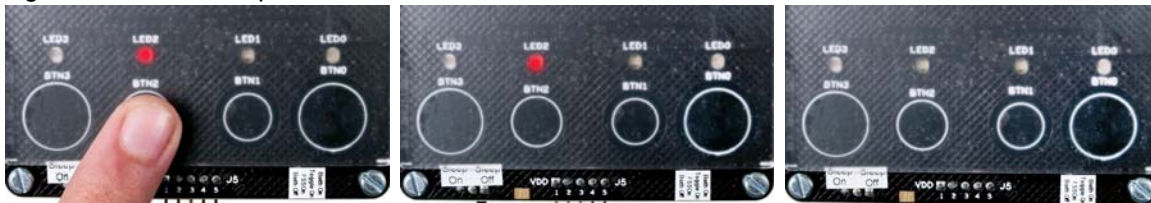
Figure 3-15. Test Sequence for LED On Time Feature
