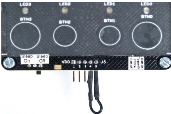
Figure 3-22. BTN1 Sensor Shorted to Ground
