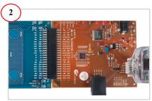
1. Connect the CY3280-SRM board to the CY3280-20x34 UCC board's P2 connector.
