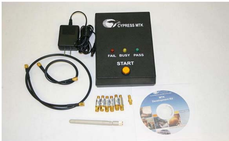
Figure 1-1. Manufacturing Test Contents
