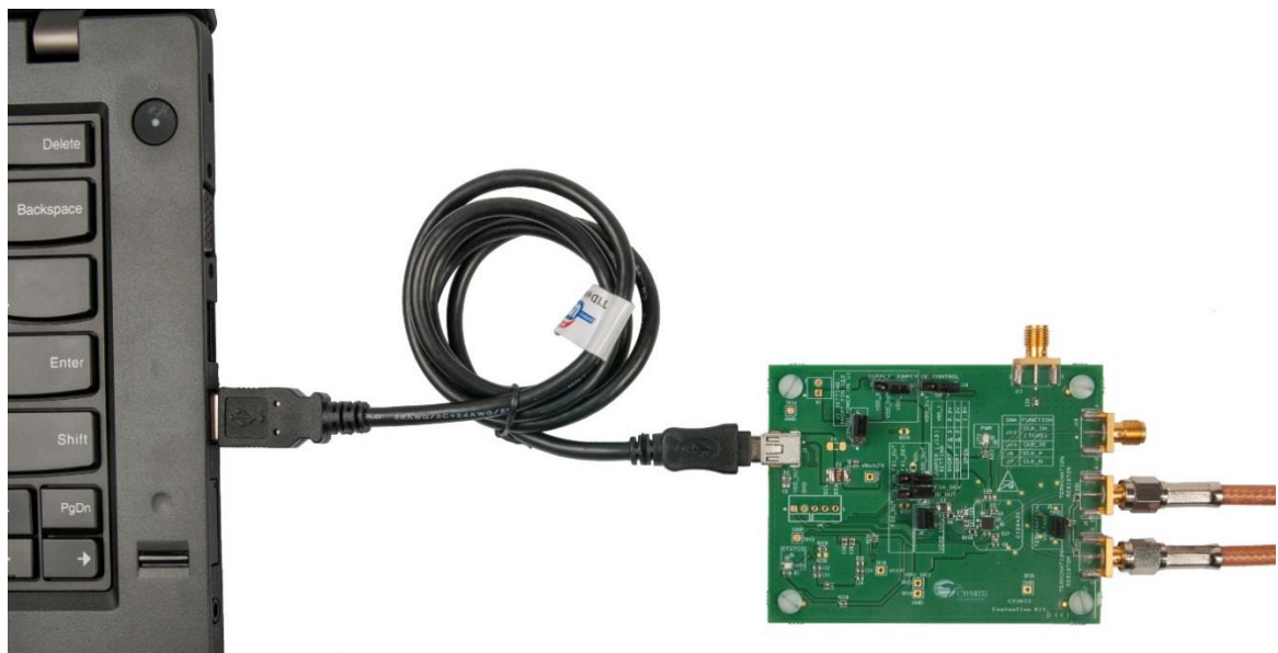
Figure 3-3. Kit Connected through USB
