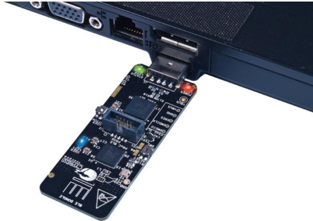
Figure 3-16. CySmart USB Dongle Connected to PC
