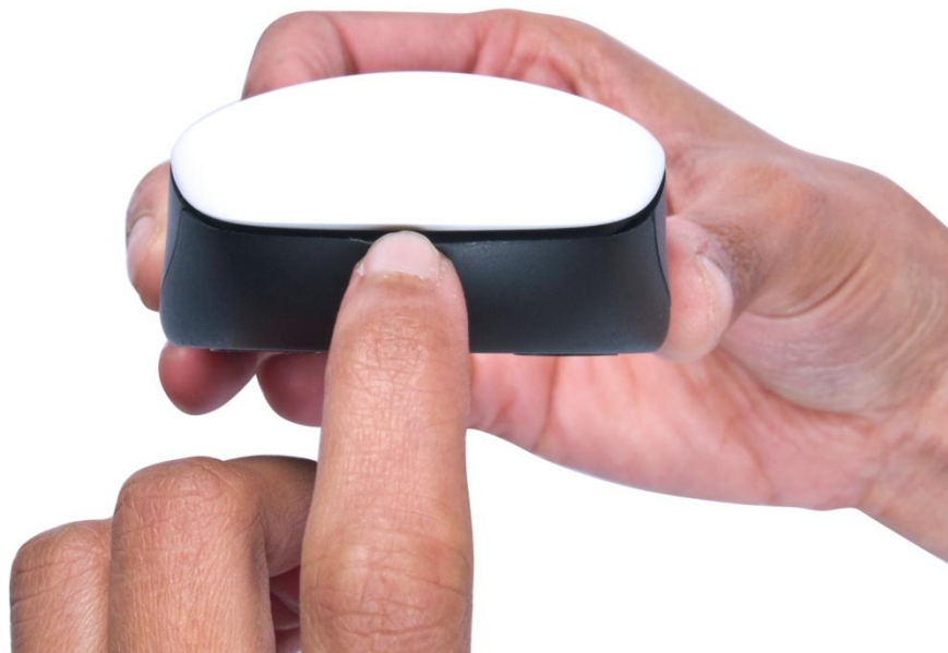
Figure 6-3. Removing the Top Cover of the Touch Mouse
