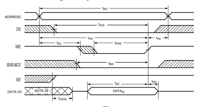
Figure 8. Write Cycle 2: CE Controlled [23, 24, 25]
