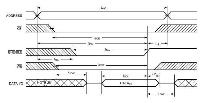
Notes 27. If  $\overline{\text{CE}}$  goes HIGH simultaneously with  $\overline{\text{WE}}$  = V<sub>IH</sub>, the output remains in a high impedance state. 28. During this period, the I/Os are in output state. Do not apply input signals.
