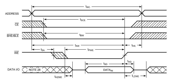
Figure 10. Write Cycle 4: BHE/BLE Controlled, OE LOW [27]
