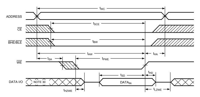
Figure 9. Write Cycle 4: BHE/BLE Controlled, OE LOW [28]
