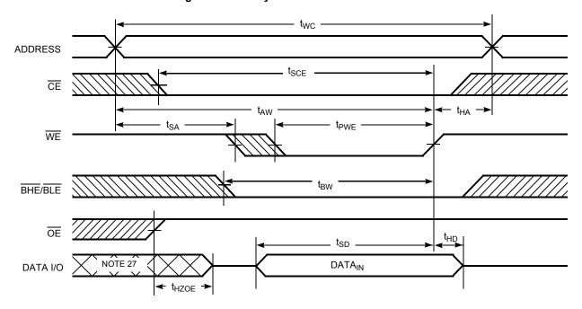
Figure 7. Write Cycle 2: CE Controlled [24, 25, 26]
