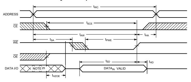
Figure 7. Write Cycle No. 2:  $\overline{\text{CE}}$  Controlled [23, 24]
