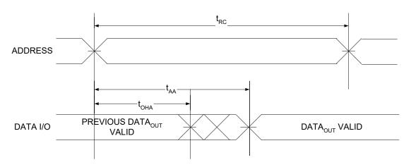
Figure 7. Read Cycle No. 2 (OE Controlled)<sup>[26, 27, 28]</sup>
