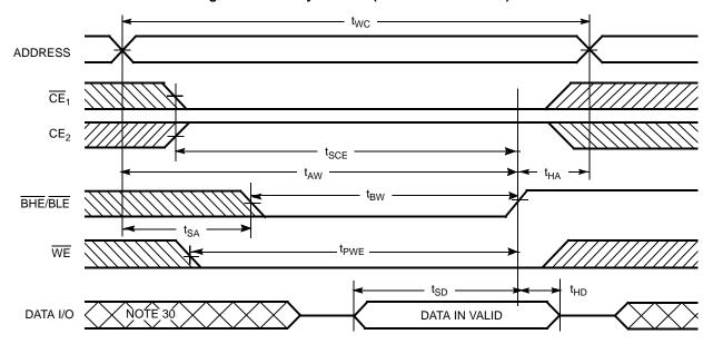
Notes 29. If  $\overline{CE}_1$  goes HIGH and  $CE_2$  goes LOW simultaneously with  $\overline{WE} = V_{IH}$ , the output remains in a high impedance state. 30. During this period the I/Os are in output state. Do not apply input signals. 31. The minimum write cycle pulse width should be equal to the sum of tSD and tHZWE.
