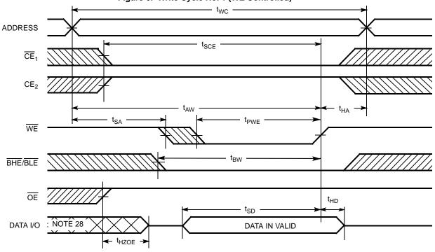
Figure 7. Write Cycle No. 2 ( $\overline{\text{CE}}_1$  or  $\text{CE}_2$  Controlled) [25, 26, 27]
