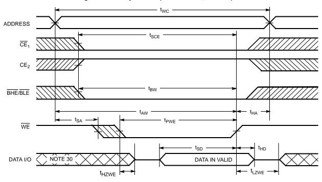
Figure 9. Write Cycle No. 4 (BHE/BLE Controlled) [29]
