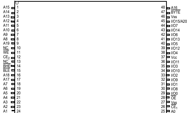
Figure 2. 48-pin TSOP I Pinout (Dual Chip Enable without ERR) – CY62167G30 [6, 7]
