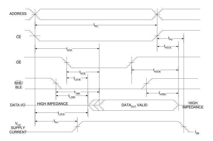
Figure 7. Read Cycle No. 2 (OE Controlled) <sup>[22, 23]</sup>
