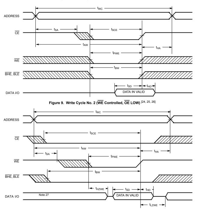
Figure 8. Write Cycle No. 1 (CE Controlled) <sup>[24, 25, 26]</sup>
