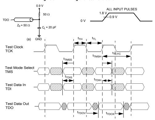
20. Test conditions are specified using the load in TAP AC Test Conditions.  $t_R/t_F$  = 1 ns.
