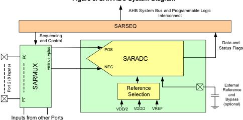
Figure 3. SAR ADC System Diagram
