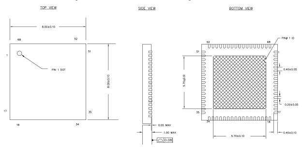
Figure 7. 68-Pin QFN 8 × 8 × 1.0 mm Package Outline
