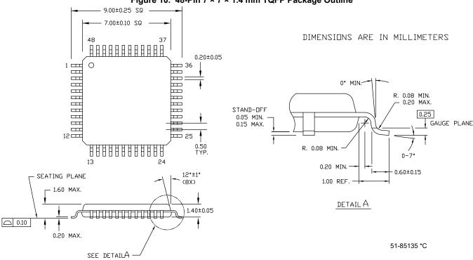
Figure 10. 48-Pin 7 × 7 × 1.4 mm TQFP Package Outline
