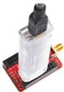
Fig-2: Programming and Debugging with CY8CKIT-002
