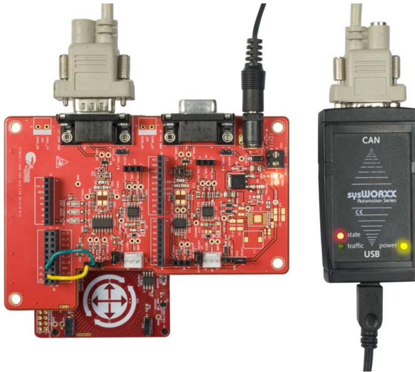
Figure 4-2. CAN Analyzer Connection to CY8CKIT-026's CAN1 Transceiver
