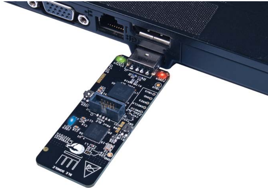
Figure 4-55. Connect BLE Dongle to USB Port
