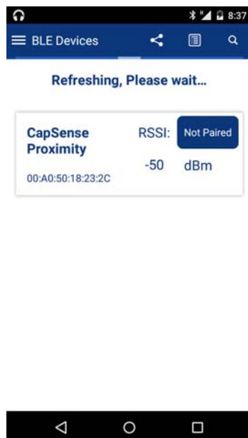
Figure 4-46. Connect to CapSense Proximity Peripheral
