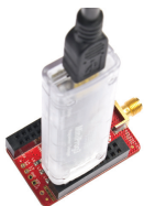
Fig-2: Programming and Debugging with CY8CKIT-002
