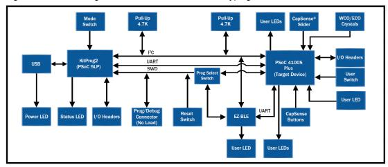
The PSoC 4100S Plus Prototyping Kit is simplistic in design and focuses on providing you with complete access to develop applications using the PSoC 4100S Plus device. This kit supports the following features:
