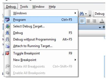
8. If the device is already acquired, programming will complete automatically and the result will appear in the PSoC Creator status bar at the bottom left side of the screen. If the device is yet to be acquired, the Select Debug Target window will appear. Select **KitProg2/<serial number>** and click **Port Acquire** as shown in Figure 4-4.
