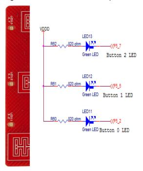
Figure A-18. Feedback LEDs for CapSense Slider
