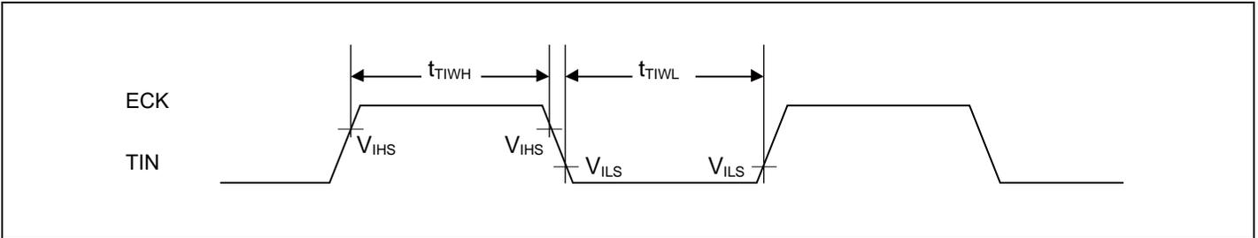
Trigger input timing
