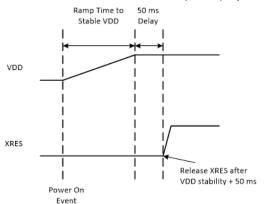
Figure 10. Power-On External Reset (XRES) Operation
