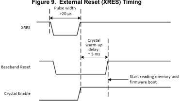
Figure 9. External Reset (XRES) Timing
