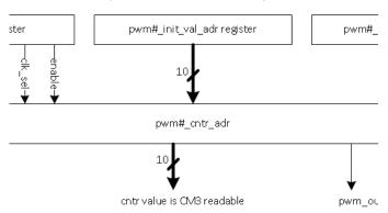
1 cntr w/pwm#\_init\_val = 0 (dashed line) cntr w/pwm#\_init\_val = x (solid line)
