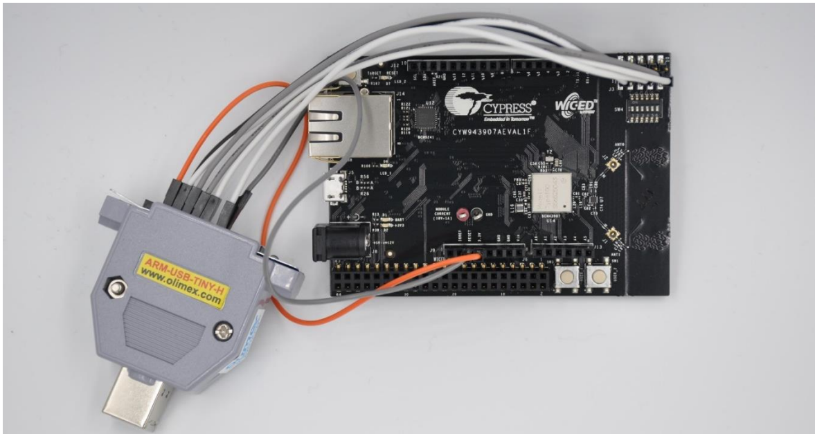
Figure 4-8. JTAG to Olimex Connection
