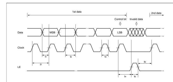
On the rising edge of the clock, one bit of data is transferred into the shift register.
