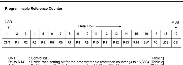
R1 to R14 : Divide ratio setting bit for the programmable reference counter (3 to 16,383) [Table 2] SW : Divide ratio setting bit for the prescaler (64/65 or 128/129) [Table 5] FC : Phase control bit for the phase comparator [Table 8] LDS : LD/fout signal select bit [Table 7] CS : Charge pump current select bit
