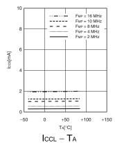
Vcc = 5.5 V,  $F_{MPL} = 16 \text{ kHz}$  (divided by 2) Subclock mode with the external clock operating
