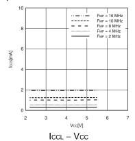
T<sub>A</sub> = +25 °C, F<sub>MPL</sub> = 16 kHz (divided by 2) Subclock mode with the external clock operating
