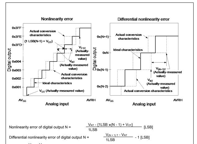
$1LSB = \frac{V_{FST} - V_{OT}}{1022}$
