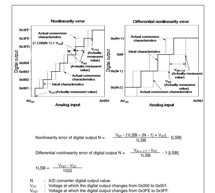
: Voltage at which the digital output changes from 0x(N - 1) to 0xN.
