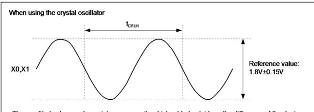
The amplitude changes by resistance, capacity which added outside or the difference of the device.
