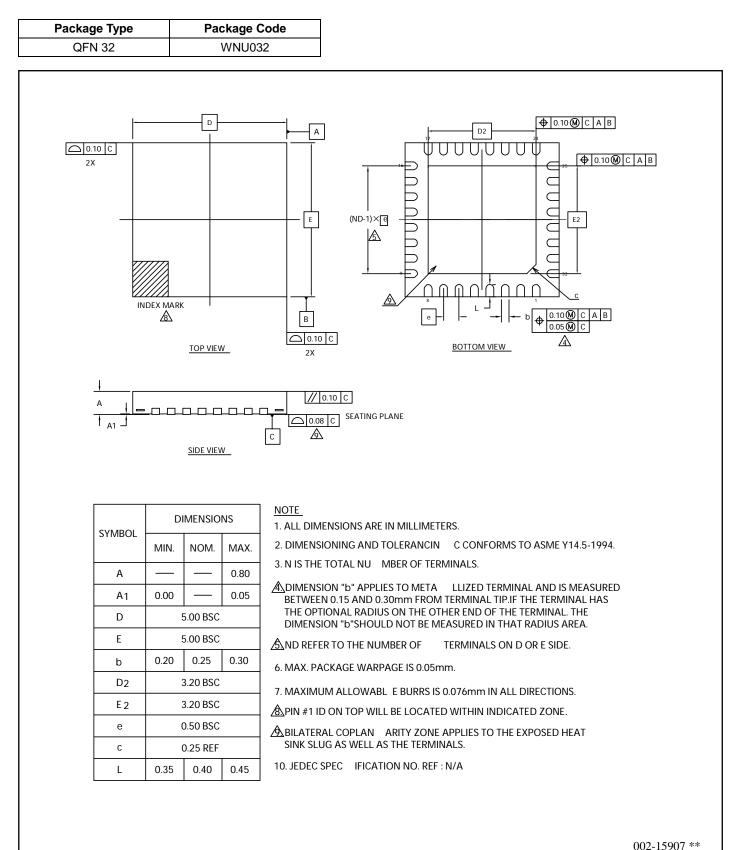
PACKAGE OUTLINE, 32 LEAD QFN 5.00K5.00K0.80 MM WNU032 3.20%.20 MMEPAD (SAWN) REV\*
