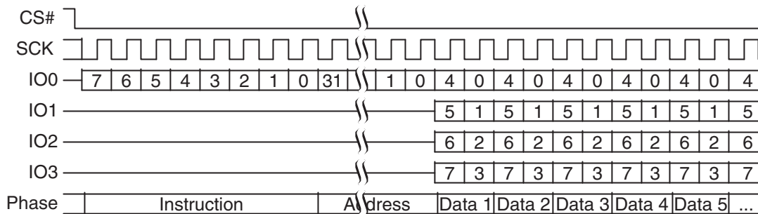
Figure 13. Quad Output Command without Latency
