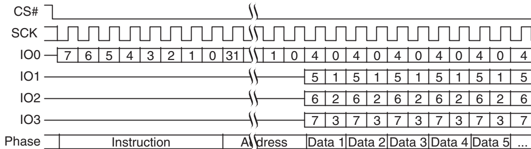
Figure 13. Quad Output Command without Latency
