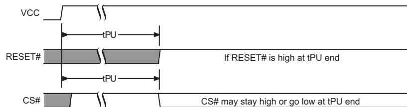
Figure 24. Reset High at the End of POR
