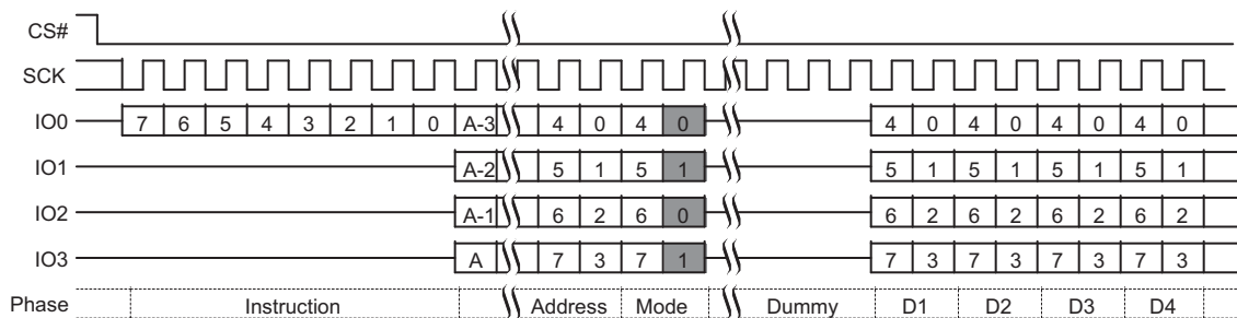
Figure 81. Quad I/O Read Command Sequence (EBh or ECh), QPI Mode [56, 57]
