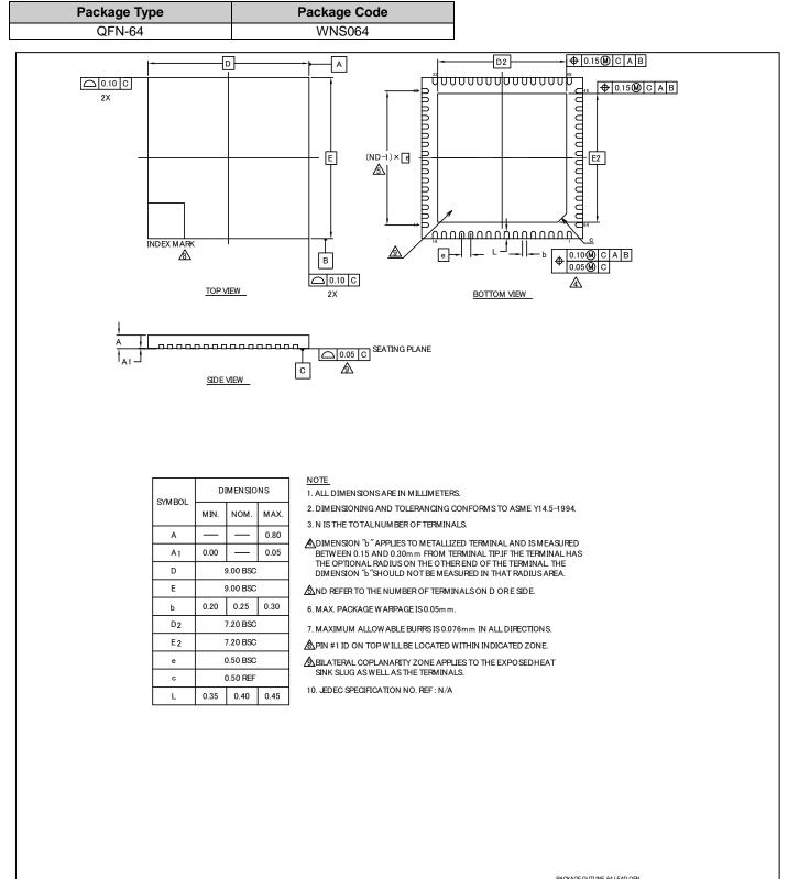
PACKAGE OUTLINE, 64 LEAD QFN 9.00X9.00X0.80 M M WNS064 7.20 X7.20 M M EPAD (SAWN) REV\*\*
