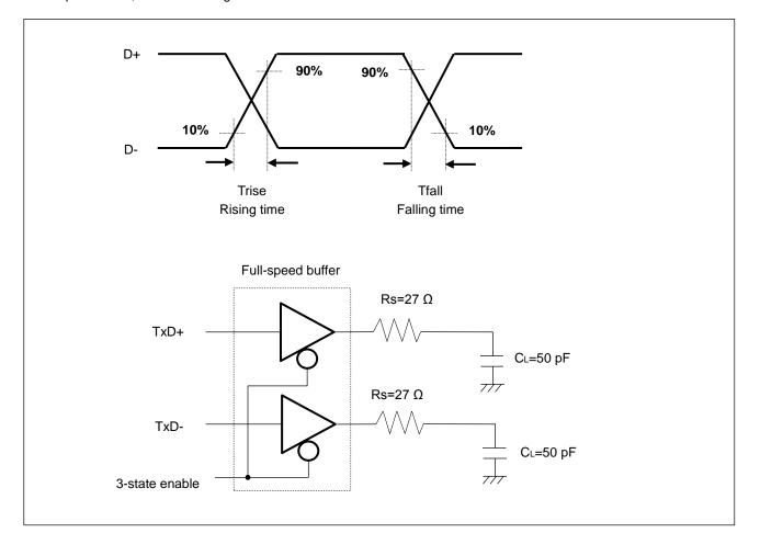
USB Full-speed connection is performed via twist pair cable shield with 90 Ω ± 15% characteristic impedance (Differential Mode).
