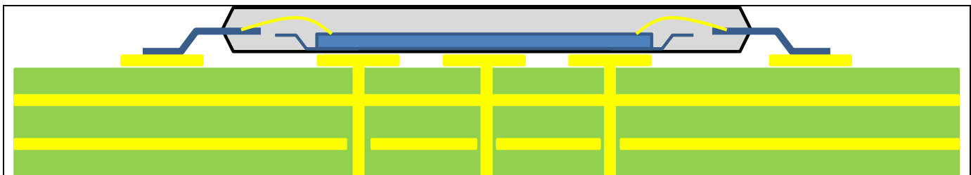
Figure 8-1: Example Thermal via Holes on PCB.
